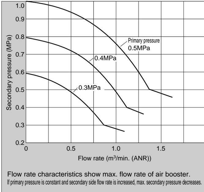
**Pressure characteristic** (Setting: Primary pressure 0.69MPa, secondary pressure 0.97MPa, flow rate 0.02m³/min. ANR)
