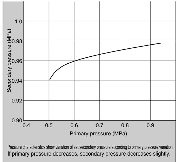
Note) Air booster needs approx. twice secondary side flow rate (max.) for primary side due to structure.
